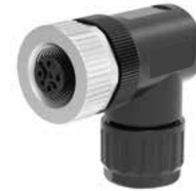
M12母弯头, 组装式(现场接线), 非屏蔽, 焊杯式 M12 Female angled connector, assembly(field), unshield, solder cup
