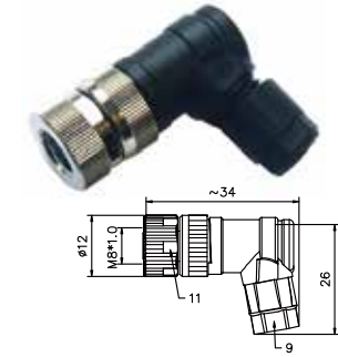
M8母弯头, 组装式(现场接线), 非屏蔽, 锁螺钉式 M8 Female angled connector, assembly(field), unshield,screw
